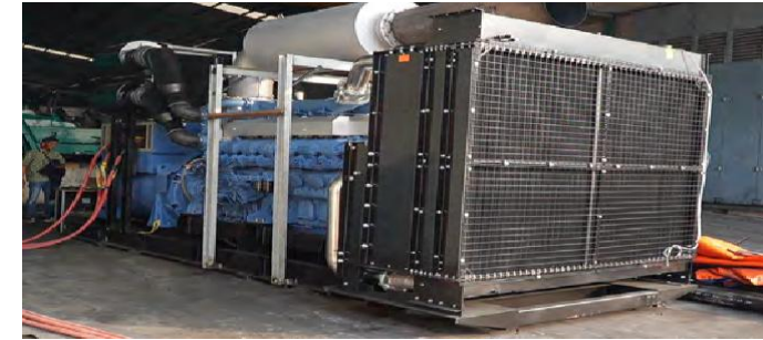
PT Pelindo - Tanjung Perak Supply (Genset) Austin Power System, Mitsubishi 2000 kVA Open 6.6 KV
